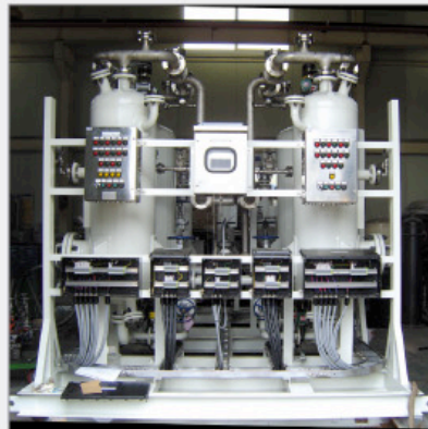
RAS LAFFAN AIR DRYER
